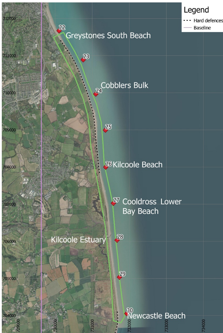
Figure A.1-3. LITLINE model extents showing baseline, hard defences (revetments), profile and nearshore wave and water level locations for CCA6.1.
