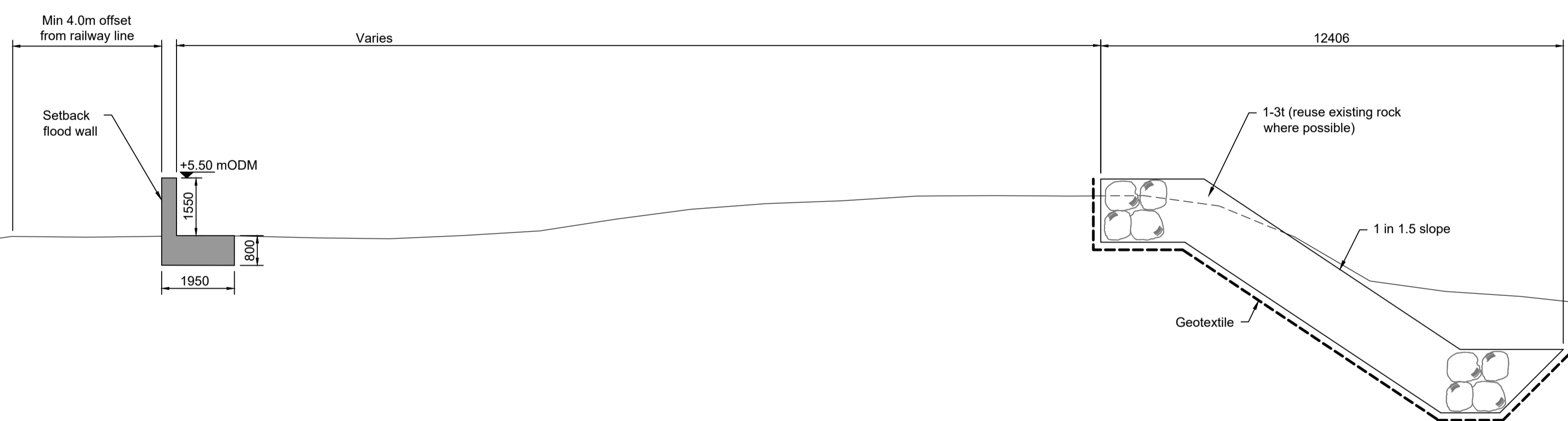
CCA6.2-C1 OPTION B - TYPICAL CROSS SECTION ROCK BERM AND SETBACK FLOODWALL Scale 1:100
