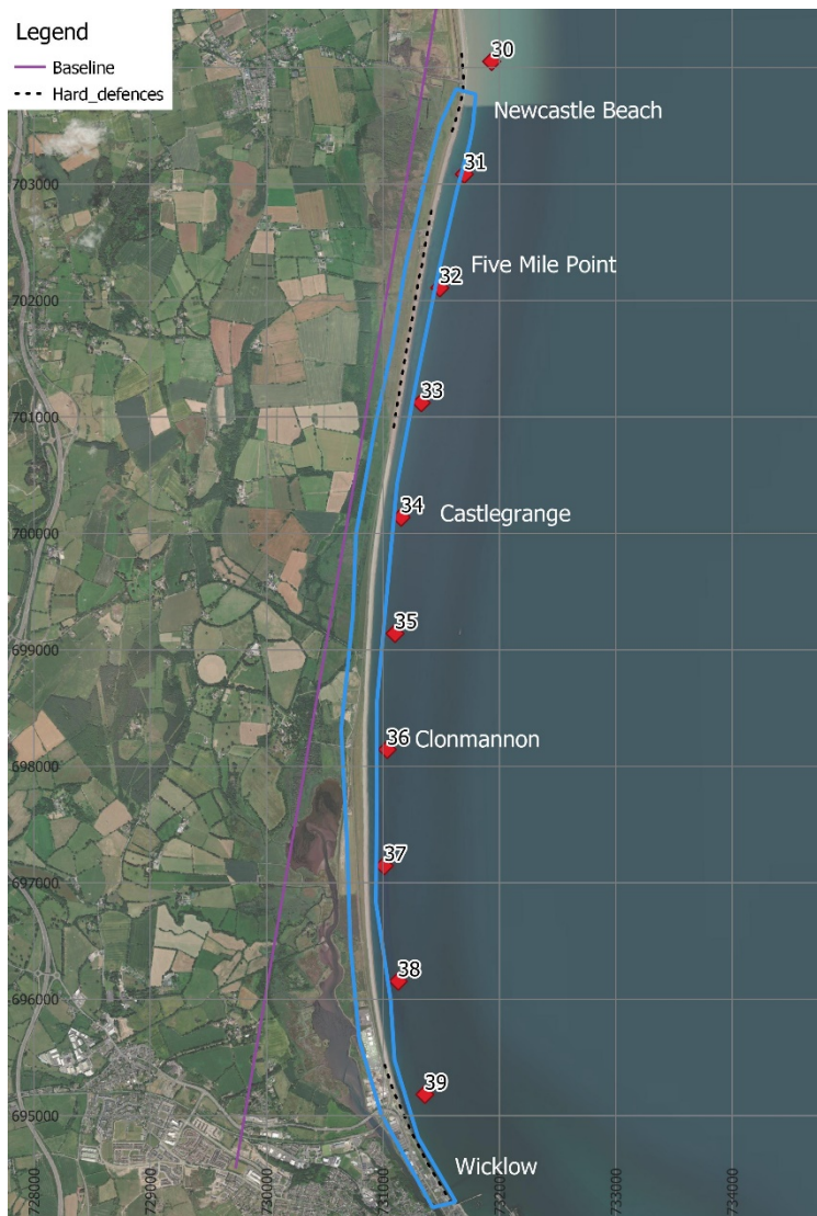
Figure A.1-3. LITLINE model extents showing baseline, hard defences (revetments), profile and nearshore wave and water level locations for CCA6.2
