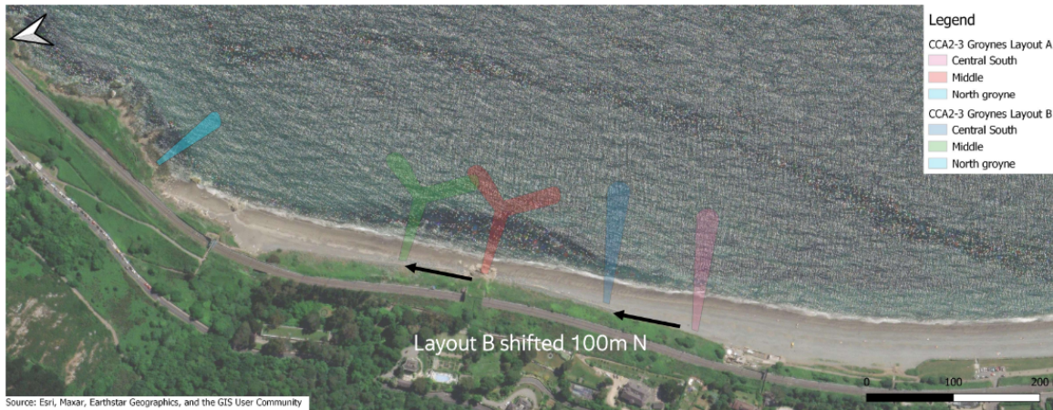
Figure A.3-10. Model layout for Groyne Layout A (in red/pink) and Layout B (in green/blue). The terminal groyne to the north is present in all layouts.
