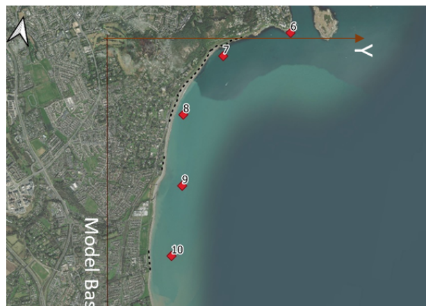
Figure A.1-1. LITLINE model extents showing baseline, hard defences (dashed line), profile and nearshore wave points (red squares) for CCA2-3
